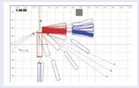
Result of an offloading simulation (wind squall).
